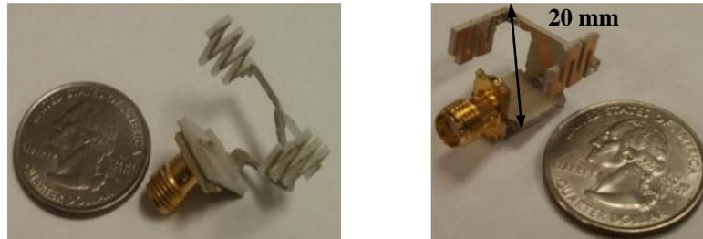
Figure 6.5: A photograph of the 3-D machined substrate cube antenna fabricated with the FDM process (left) and fabricated with the PCB technology (right).
